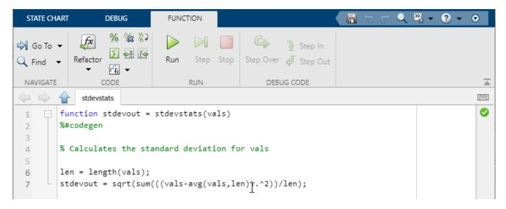
To open the editor, in a Stateflow chart, double-click a MATLAB Function block. The **Function** tab opens and the canvas shows the MATLAB function. To navigate back to the chart, use the navigation
