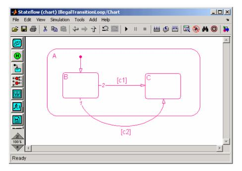
In this chart, transition 1 loops outside of logical parent A, which is the common parent of transition source B and destination C.
